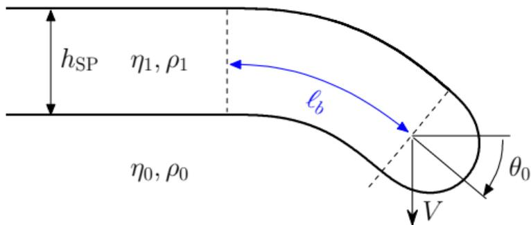
Viscous dissipation within the SP
