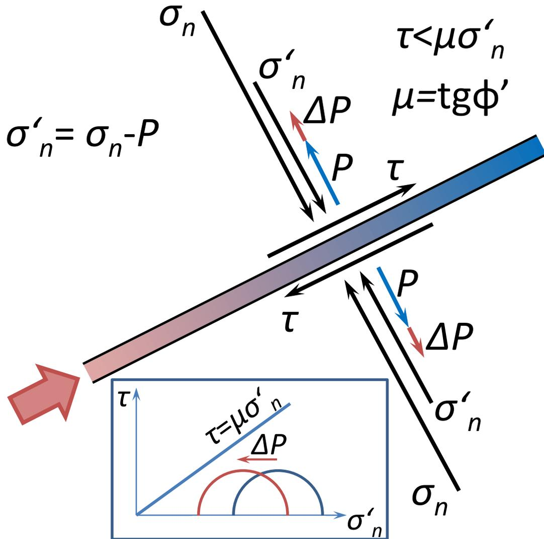
Fluid injection produces a pore pressure increase ( $\Delta P$ ) inducing fluid flow through the fracture.
