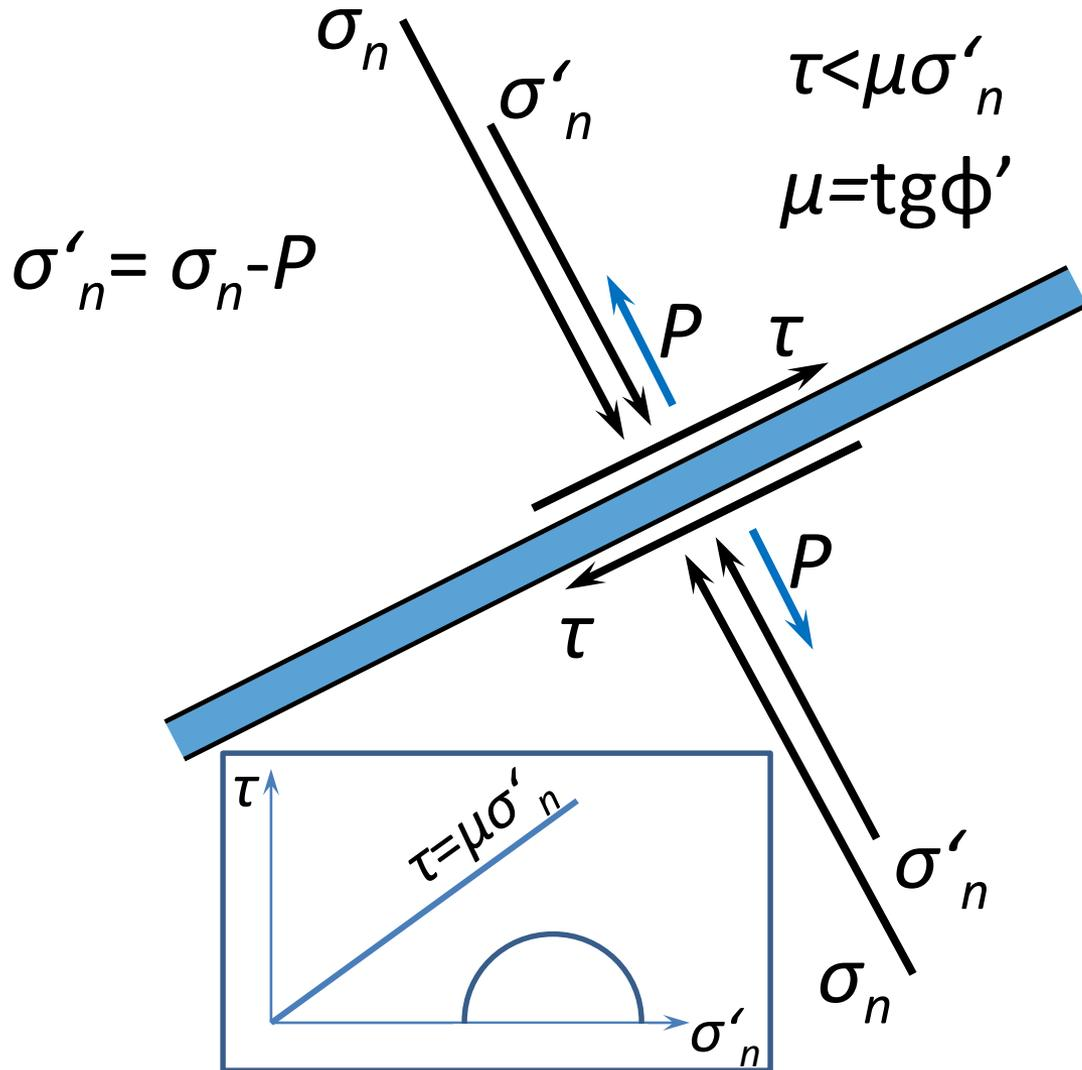
A fracture is stable while tangential forces ( $\tau$ ) are lower than the friction coefficient ( $\mu$ ) multiplied by the fracture normal effective stress ( $\sigma'_n$ )
