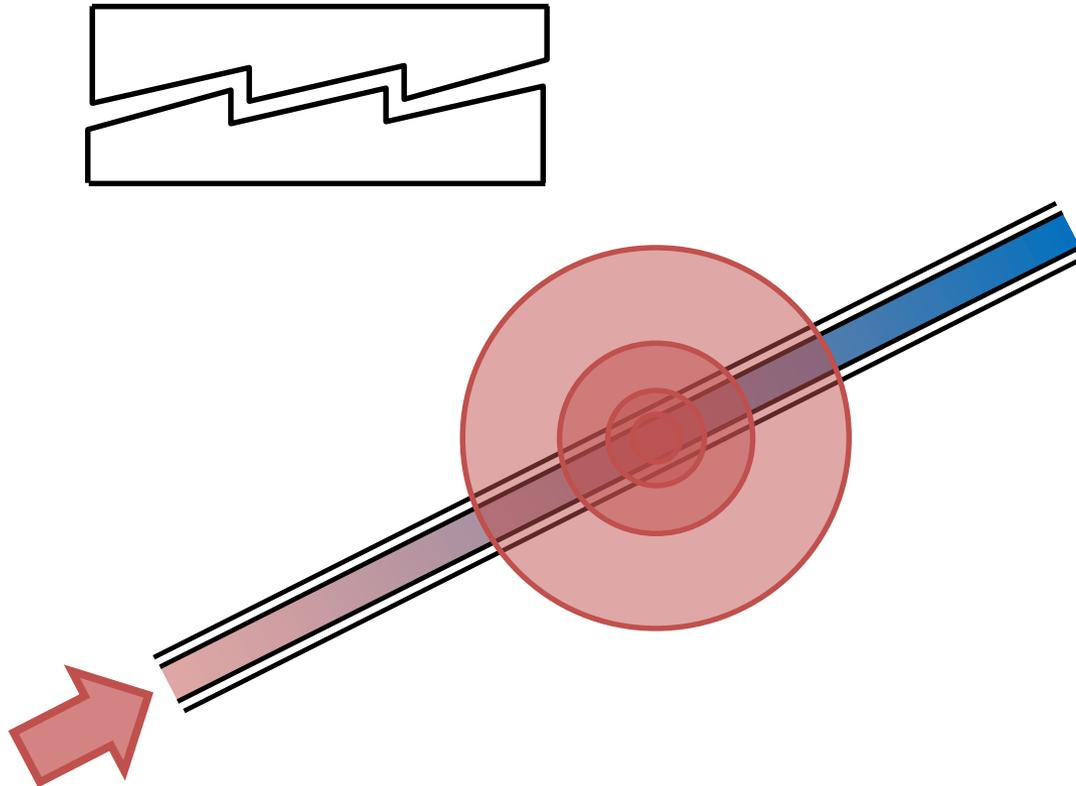
Sliding will open the fracture and trigger a microseismic event.
