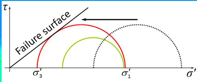
Since horizontal stress does not increase in the lower half of the reservoir, the deviatoric stress is maintained, becoming the most critical zone
