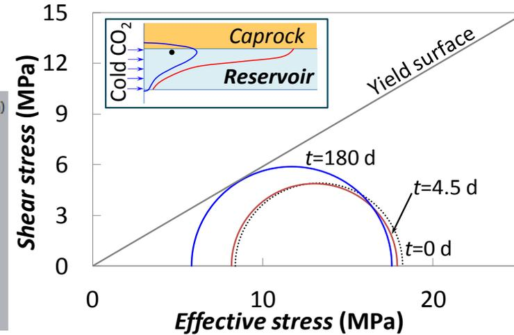
This causes a stress redistribution to satisfy stress equilibrium and displacement compatibility that tightens the lower portion of the caprock (**caprock integrity is maintained**)
