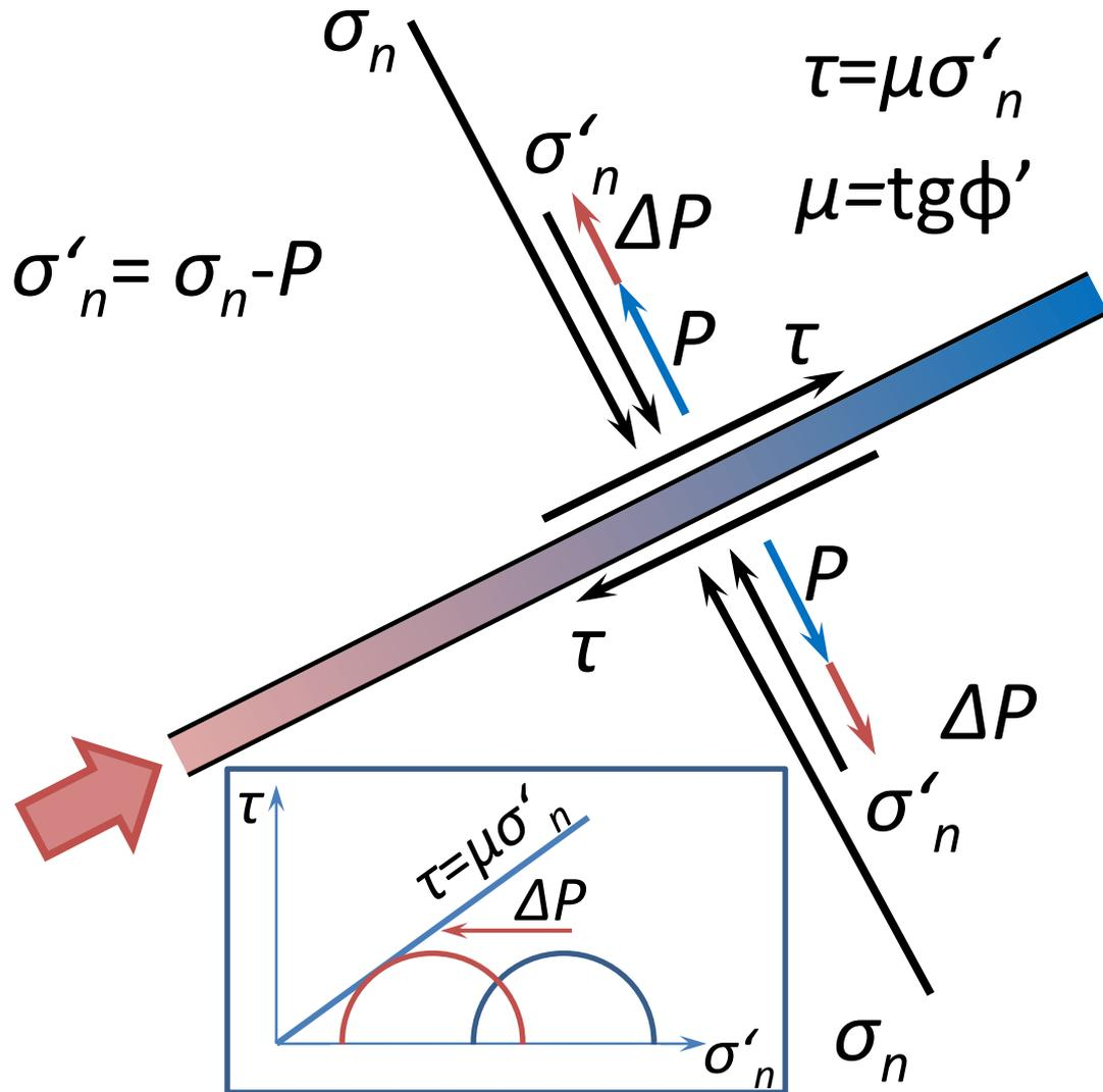
If the overpressure ( $\Delta P$ ) is high enough ( $\tau = \mu \sigma'_n$ ), shear slip occurs between the planes of the fracture
