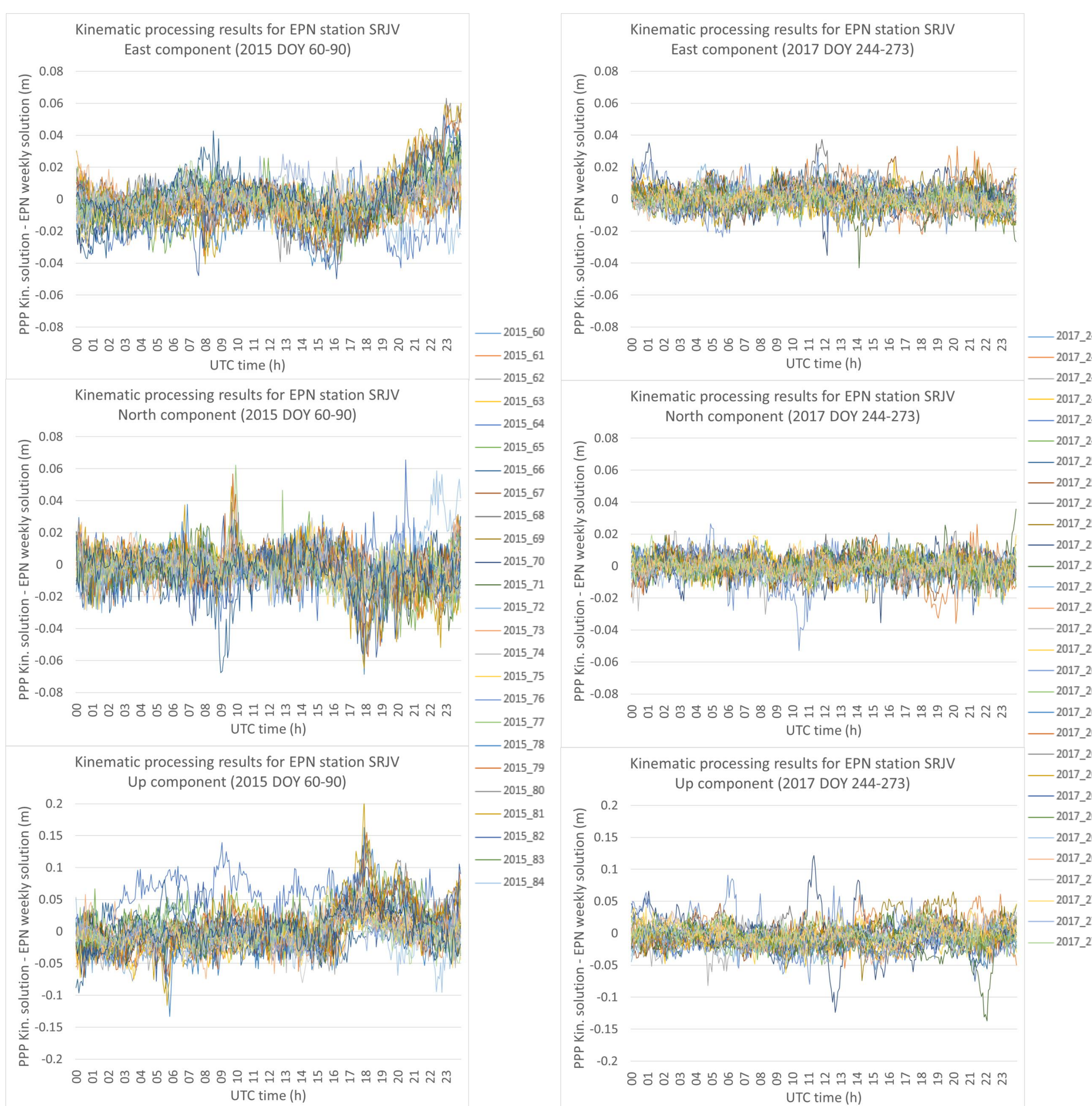
Fig.4: Hourly kinematic processing results in ENU components - PPP Kinematic solution minus EPN weekly solution (left: March 2015, right: September 2017). Higher differences during the day are noticeable for the period of March 2015 (max. 0,22 m in Up component) compared to September 2017 (max. 0,13 m in Up component).
