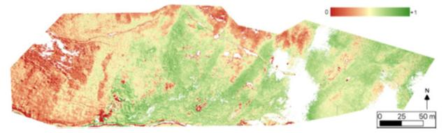
Fig. 8 UAV-based Normalised Vegetation Red Edge index (NDRE) - vegetation vitality
