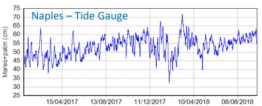
Sea level changes measured by BPR (Buoy CFBB) have been divided for density of the sea water and gravitational acceleration. Than we use the Naples Tide Gauge, **located outside the deformation area**, as stable reference
