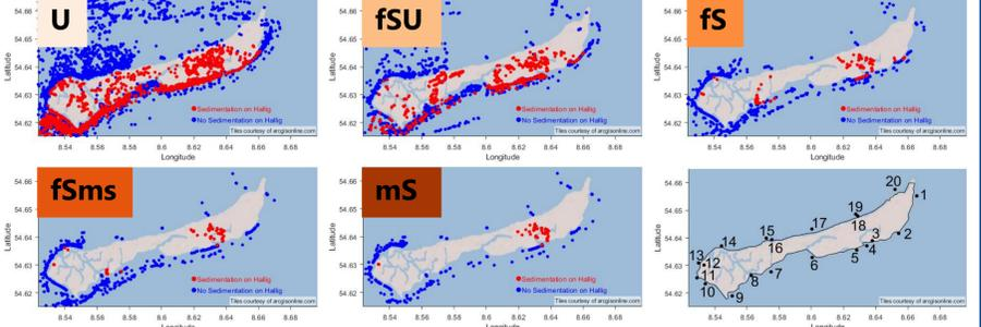
**↑C I:** Particle tracks indicating whether the individual particles sediment on (red) or off (blue) the Hallig Langeneß. Each figure shows the tracks for one of the considered grain sizes (see B III). The shown event is the storm surge "Xaver" on 6<sup>th</sup> December, 2013.
