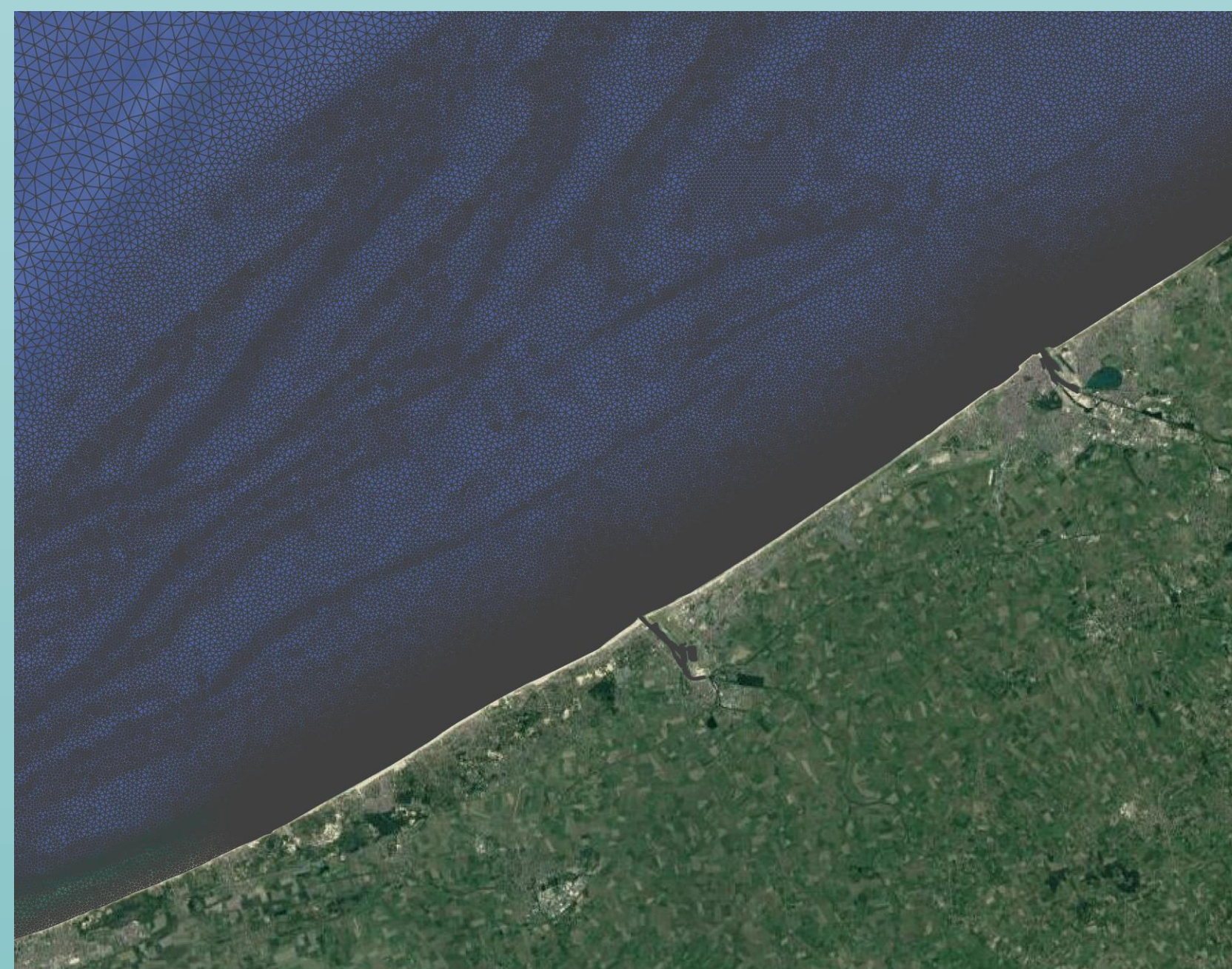
Part of the computational grid of Scaldis-Coast model where the element size is adapted to the bathymetric slopes of the existing sand banks of the Belgian coast.
