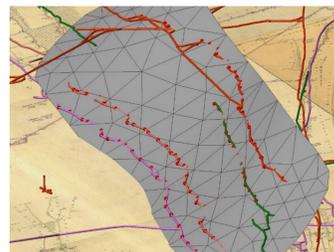
Fig.3: Fault surfaces created by discrete smooth interpolation on tunnel drifts used as constraints.
