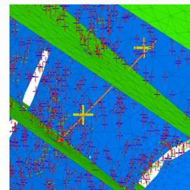
Fig.8: Top view of small model stress field. Up is direction of  $\sigma_H$ . Orange is injection well path, yellow are markers of frac intervals and corresponding histogram position for stress magnitude inside model. Stress tensors show direction of maximum compressive stress (red) is parallel to  $\sigma_H$ . Direction of intermediate stress matches vertical stress. For calculation we fixed the locally mapped faults (green) as they would perturb calculated stress directions and magnitudes.
