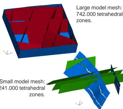
Fig.6: Discontinuities in meshes for numerical modeling performed with DEM code 3DEC by ITASCA. Large mesh extended with auxiliary blocks parallel to regional principal stress directions. Meshes generated in RHINO with GRIDDLE plug-in.
