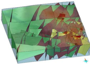
Fig.4: Large scale 3D model covers 2.5 x 2.5 x 0.5 km and contains topography, tunnels and 45 fault structures.
