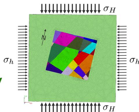
Fig.7: Top view of large numerical model with total extent 5 x 5 km. Model parameters from core tests. Stress boundary conditions. Bottom fixed in z-direction. Initial stress ratio 0.7 : 1. Large model results used as boundary stress to smaller integrated model.
