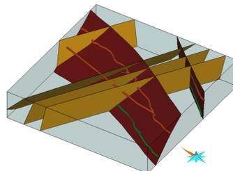
Fig.5: Small scale integrated model. Includes tunnel drifts, boreholes and locally mapped fault structures (yellow). 250 x 250 x 50 m.
