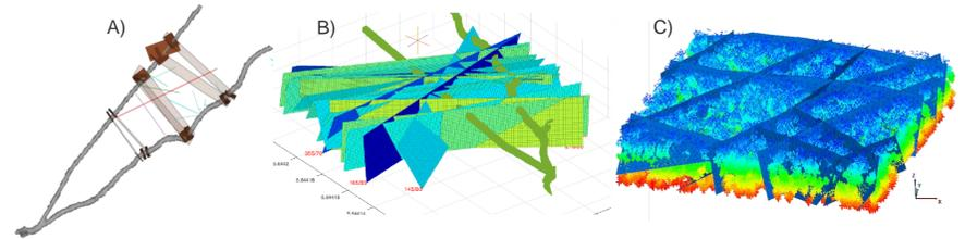
Fig.1: Different stages of the modelling process. A) 3D model representation of the test site with tunnels obtained from 3D laser scans (MABB), boreholes and mapped fault structures. B) Preceding slip tendency analysis of mapped fault structures at test site. C) Stress field model based on large 3D geomodel.
