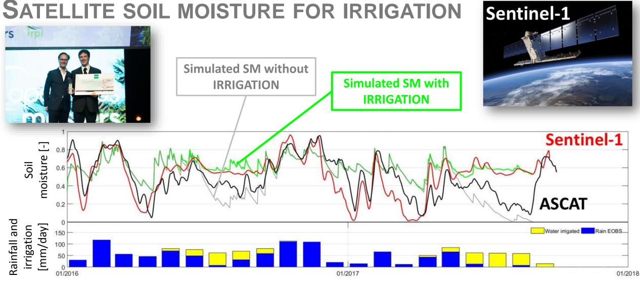
**Sentinel-1 (S1)** seems to be able to see the irrigation signal at small spatial scale, differently from coarse resolution ASCAT soil moisture.
