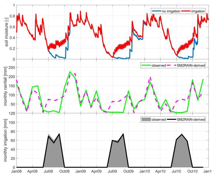
We simulate soil moisture without (blue line) and with (red line) irrigation
