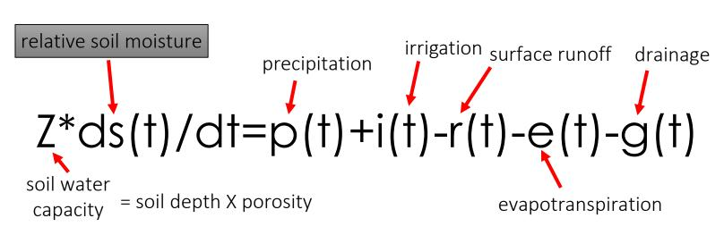
Inverting the water balance equation for i(t), assuming:
