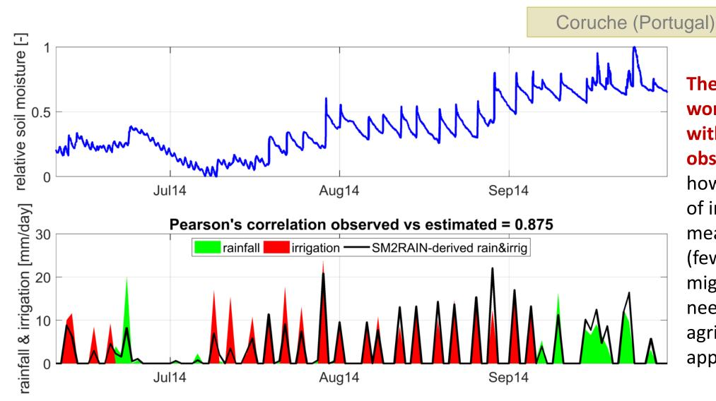
The method works very well with in situ observations, however the scale of in situ measurements (few meters) might not fit the need of agricultural applications
