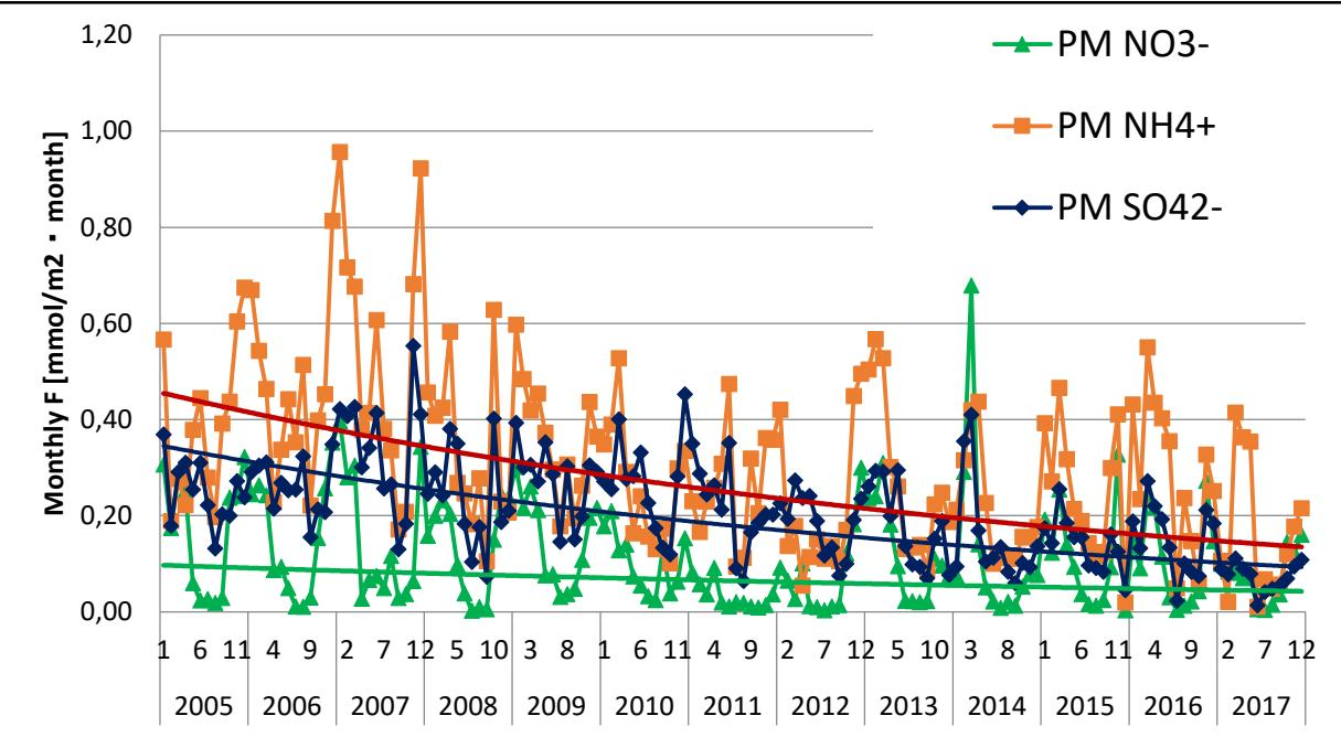
Monthly values of dry deposition flux of PM  $\text{NO}_3^-$ ,  $\text{NH}_4^+$ ,  $\text{SO}_4^{2-}$
