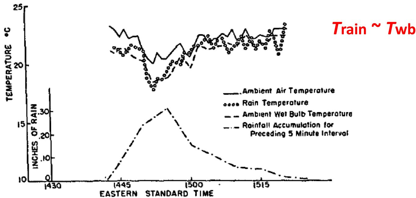
FIG. 6. Air-rain temperature relationships, Type I; 14 August 1947, Station B, Clinton County Air Force Base, Wilmington, Ohio.
