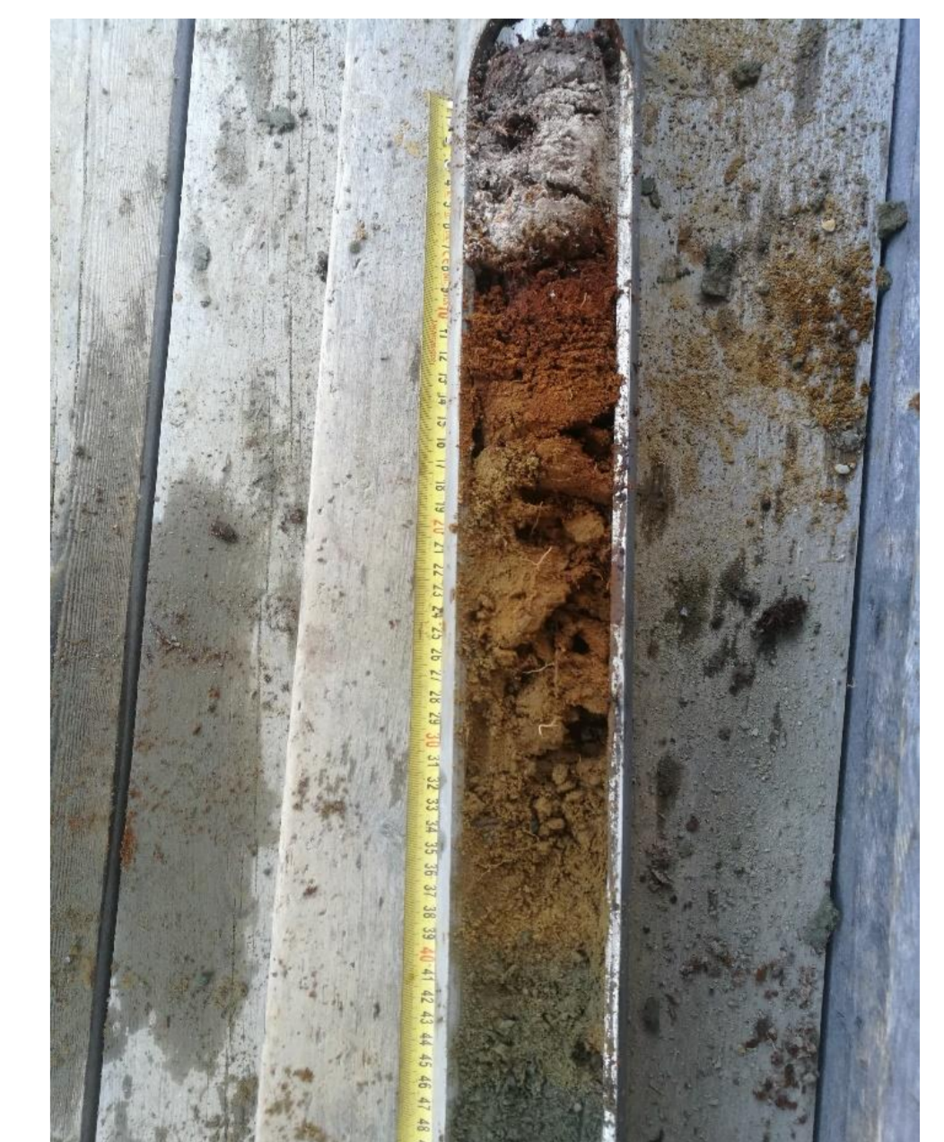
Figure 7. Window sampler with podsol soil from the experimental plot
