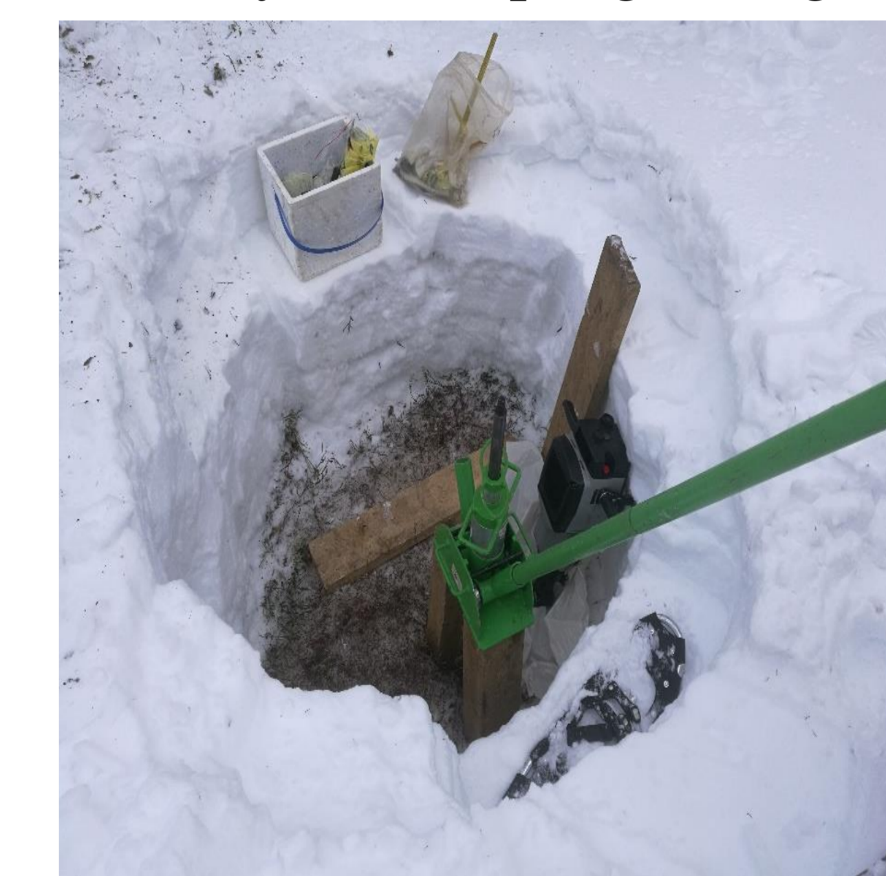
Figure 6. Extracting soil core in winter conditions
