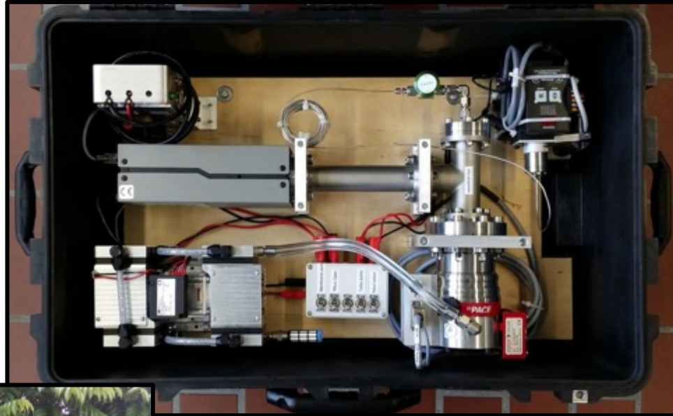
Above: miniRUEDI mass spectrometer including pumps, electronics and switching valve to measure from different ports. Left and right: MiniRUEDI during operation in field.
