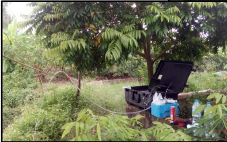
Above: miniRUEDI mass spectrometer including pumps, electronics and switching valve to measure from different ports. Left and right: MiniRUEDI during operation in field.
