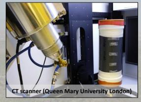
Method: X-Ray Computed Tomography (X-Ray CT) combines the penetrating capacity of X-rays with 3D-volume reconstruction to observe the internal structure of objects in a non-destructive manner. Frequently used in agricultural science, it also offers an unprecedented opportunity to observe the more diverse subsurface environment of a saltmarsh.
