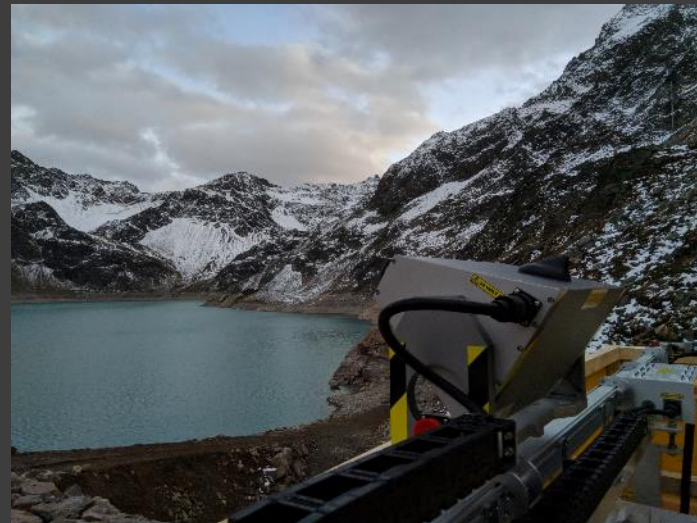
Figure 5: Radar-antenna of the GB-InSAR installed at the Finstertal reservoir in October 2019.
