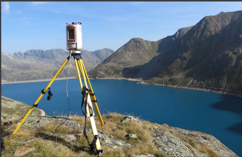
Figure 4: Terrestrial laser scanning was performed annually since 2006 from several scan positions around the reservoir.
