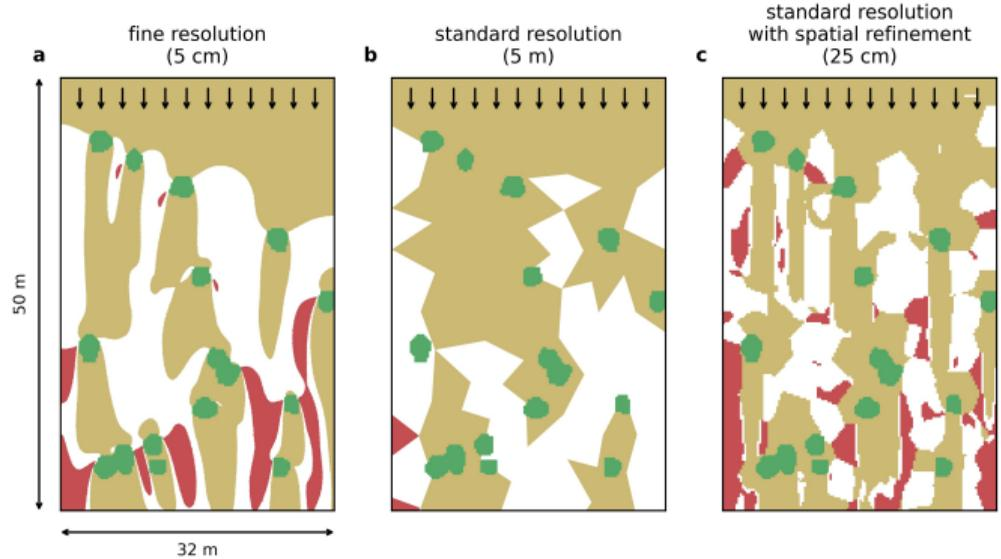
Zones of potential plant growth (yellowish) and of potential channel incision (red) resulting from flow velocities around vegetation patches (green) simulated at (a) fine-resolution, (b) standard-resolution and (c) standard-resolution with application of our new spatial-refinement method.
