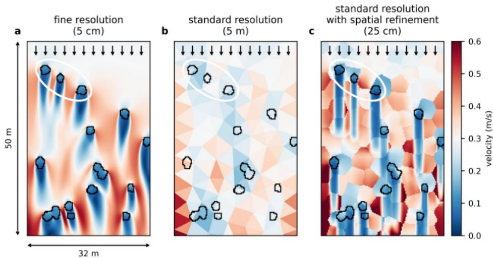
Flow velocities around vegetation patches simulated at (a) fine-resolution, (b) standard-resolution and (c) standard-resolution with application of our new spatial-refinement method. The black lines represent the contour of the vegetation patches. The single-headed arrows indicate the incoming flow direction and the double-headed arrows the domain dimensions.
