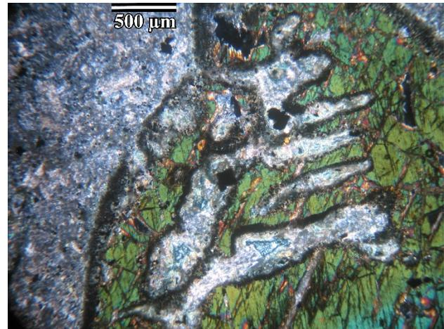
Magmatically corroded amphibole
