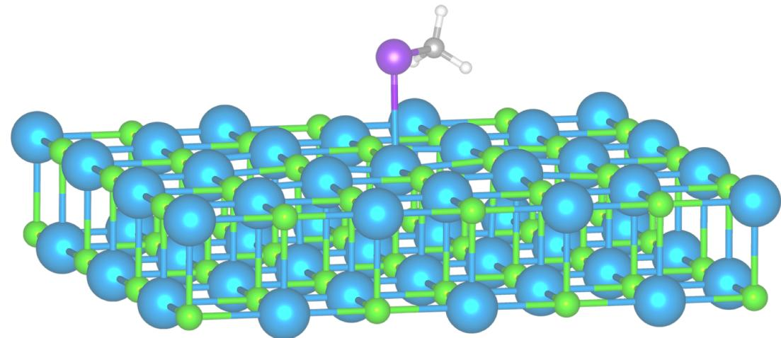
*Optimized DFT geometry of CH<sub>3</sub>I adsorbed on a NaCl(100) surface from a QM/QM' ONIOM (DFT/PM7) calculation*
