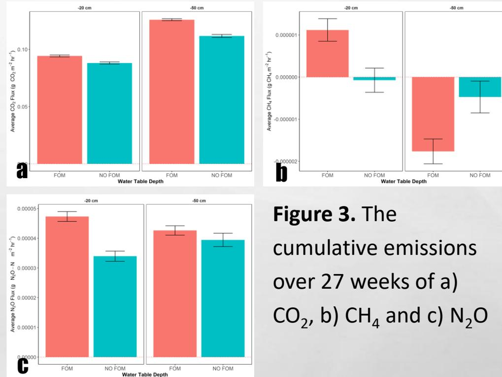
**Figure 3.** The cumulative emissions over 27 weeks of a) CO<sub>2</sub>, b) CH<sub>4</sub> and c) N<sub>2</sub>O
