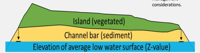
Vegetated island atop sedimentary bar and low water surface (z-value) for calculating island volume
