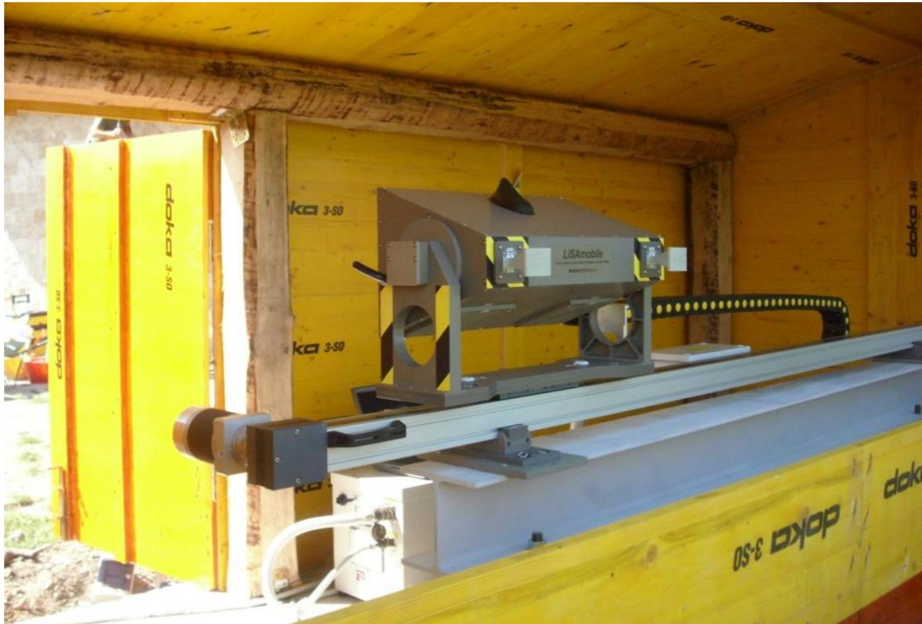
Modern GB-InSAR apparatuses, capable of acquiring in less than one minute, enable the early warning of rigid (brittle) rock failures
