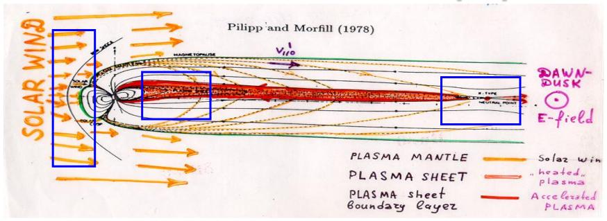
Thin current sheets in planetary magnetospheres can be formed due to interaction of <u>ANISOTROPIC p</u>lasma streams from northern/southern plasma mantles
