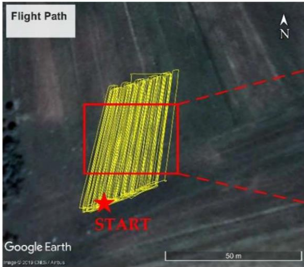
Figure 9. The planning of test site and flight path, multiple parallel profiles along the south-north direction cover the test area. The “START” is the starting point of the drone in the experiment and the trimmed profiles in the local coordinate are given on the right.
