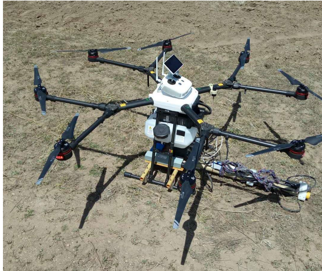
Figure 2. The UAV-magnetometer system. Notice that the boom is half-fixed.
