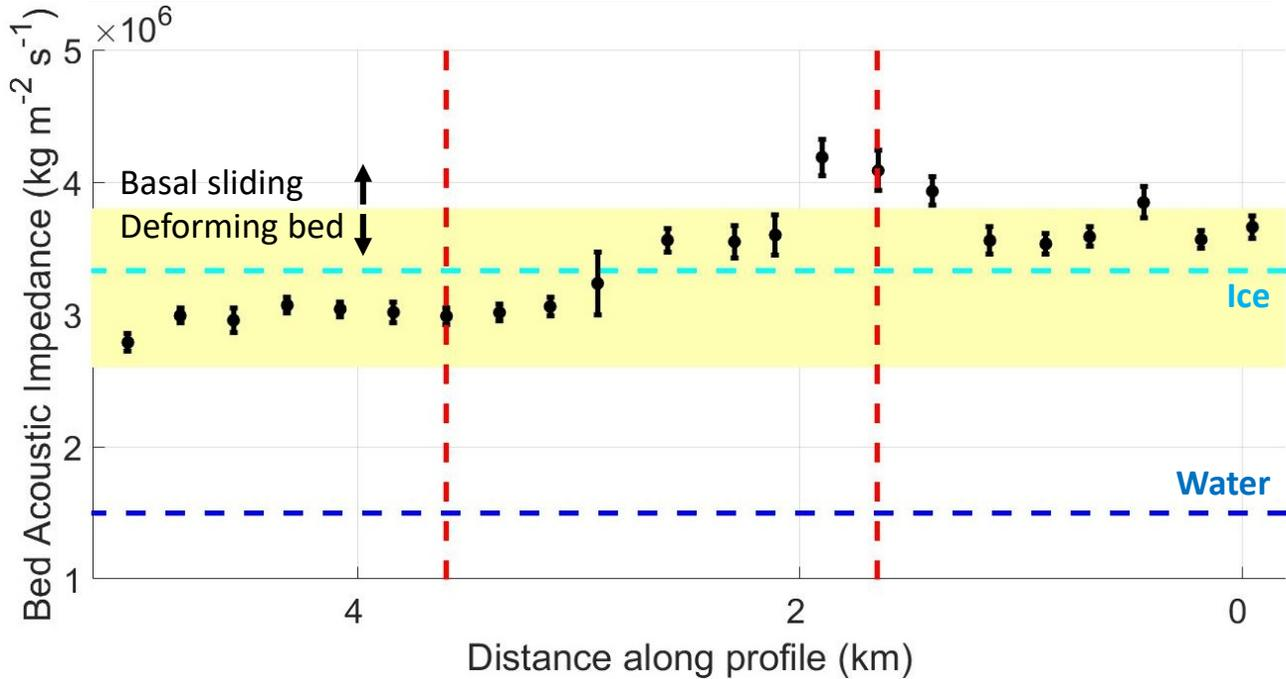
Calculation of shot size and estimated seismic properties of ice allows calculation of basal acoustic impedance from reflection strength (Holland & Anandakrishnan, 2009)
