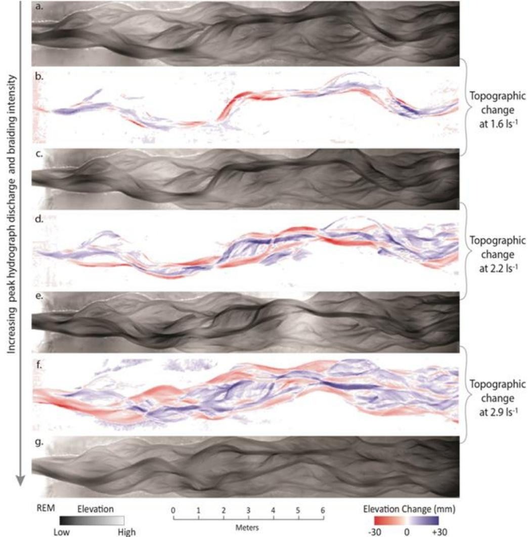
A morphologically active gravel river bed (braided in this case) undergoes constant morphological change at mobilising flows. This can be seen as intricate patterns of positive and negative elevation change over a defined time period (minutes in this case of active braiding in a flume)
