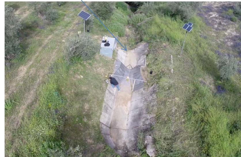
Figure 2. Equipment at the outlet to measure rainfall-runoff-sediment load. (Measurements since April 2005-April-2016)
