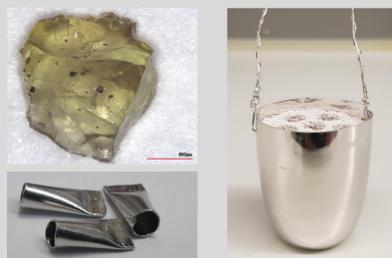
The olivine grains are handpicked and as basalt free as possible and put individually in Pt crucibles contained in a Pt basket.
