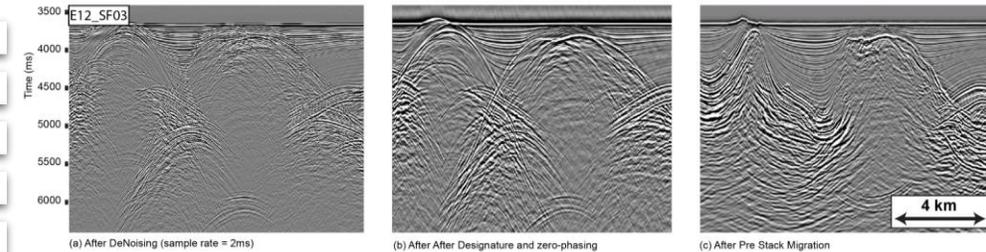
Part of stacked sections of line E12\_SF03 through the different processing steps. Bandwidth enhancement using deghosting, water-bottom derived designature and zero-phasing allow to effectively boost the low-frequency content of the data. The base of the salt structure appears more clearly
