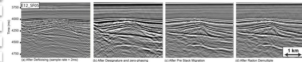
Part of stacked sections of line E12\_SF05 through the different processing steps. Locally, peg-leg multiples are hiding the signal below the salt unit. A first attempt to filter them in Radon domain by exploiting their move-out difference does not remove them completely (notice the residual peg leg of top-salt) because their velocity is too close to the primary signal.
