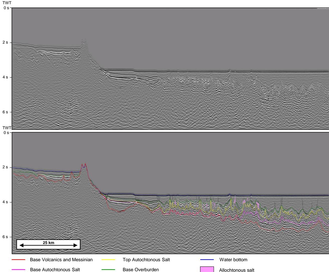
New interpretation of the Pre-stack Migrated profile SALTFLU-09 (AE12\_SF09). The new images display a better resolution of the salt structures edges and new reflectors below the salt. New interpreted thickness suggest a thicker Messinian upper Unit, a much thinner Mobile Unit, and a possibly thicker Lower Unit at the center of the Algero-Balearic abyssal plain. The interpreted horizons will be used to build the initial model for depth processing. Vertical exaggeration x4.
