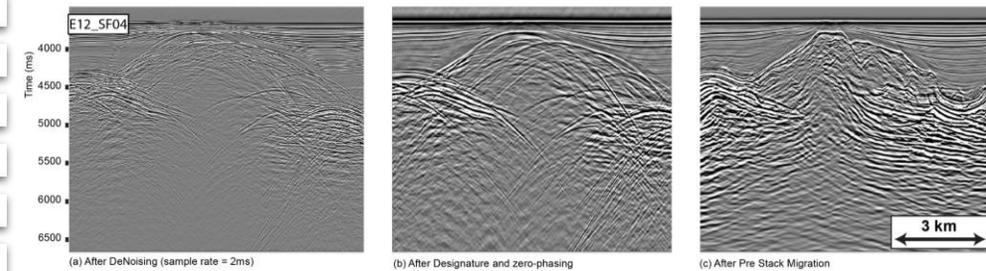
Part of stacked sections of line E12\_SF04 through the different processing steps. A 3km interval picking grid has improved the results of migration, revealing reflections below the salt. Further work to remove out-of plane reflections and, more importantly, pre-stack depth migration will improve the output images
