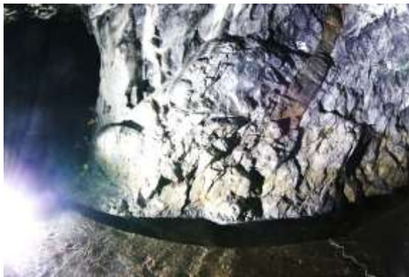
Figure 2. The wall of the underground mine. The wall material is marble, the dark vein is amphibolite.
