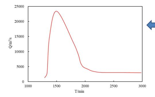
Outburst flood hydrograph measured by a hydrologic station 168 km downstream of the Sedongpu dam
