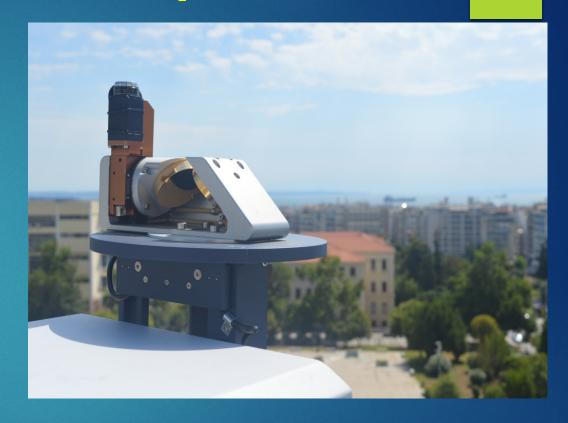
It consists of a spectrometer body with dimensions of 35x40x27cm and a solar tracker directly mounted on the spectrometer. It weighs approximately 25 kg and its design achieves high stability and is resistant to thermal influences and mechanical disturbances.
