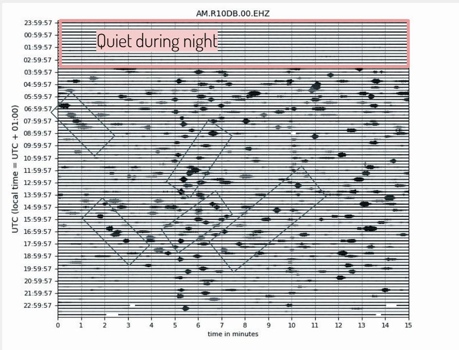
This is how a day of our example seismic station (Raspberry Shake R10DB) looks like. The helicorder plot shows the regular patterns during the day..
