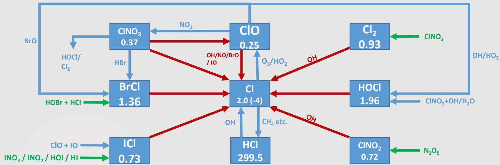
Masses in the boxes are in Gg Br. Chemical pathways are in blue, photolysis reactions are shown in red and heterogeneous ones in green.
