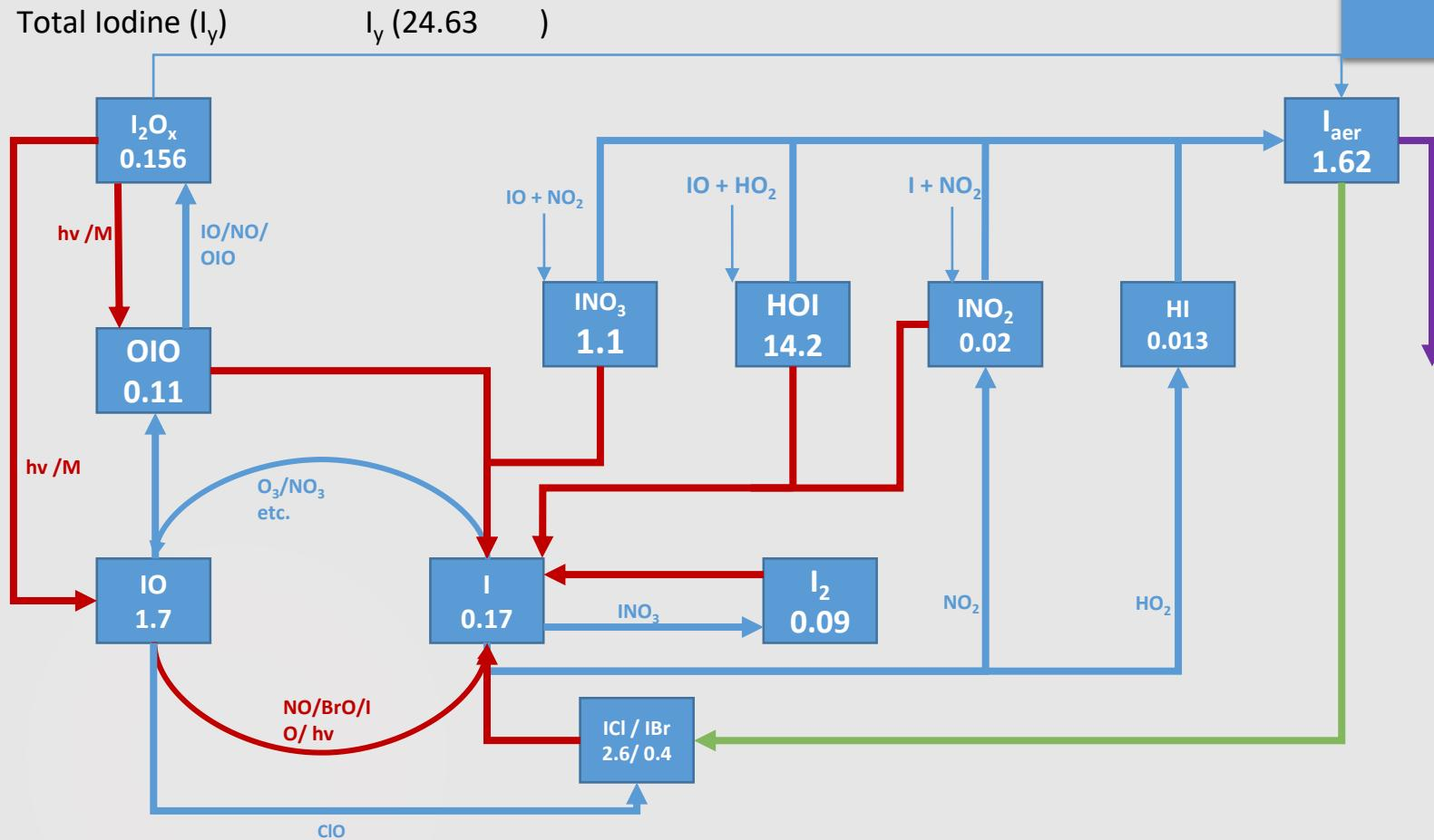
Masses in boxes are in Gg I. Red lines for photolysis; blue lines for chemical pathways; green lines for heterogeneous pathway; purple lines, depositional pathway.
