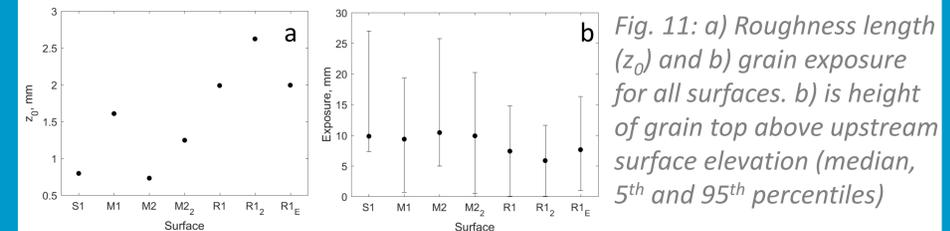
Fig. 11: a) Roughness length ( $z_0$ ) and b) grain exposure for all surfaces. b) is height of grain top above upstream surface elevation (median, 5th and 95th percentiles)
