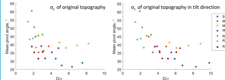
Fig. 6: Mean pivot angles against  $D/\sigma_z$  and  $D/\sigma_z$  calculated in the tilt direction.
