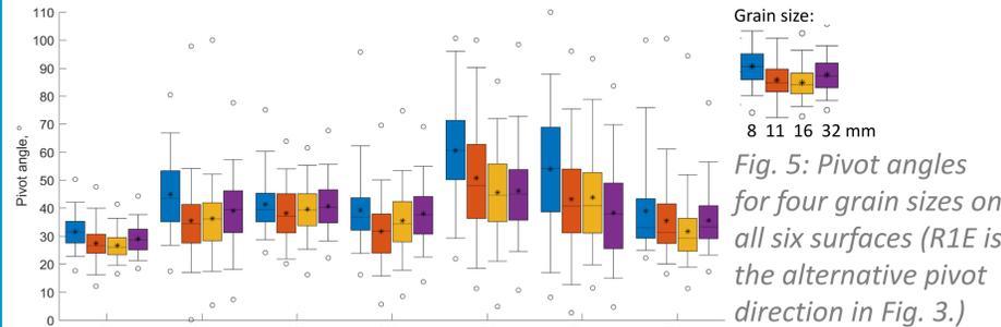
Fig. 5: Pivot angles for four grain sizes on all six surfaces (R1E is the alternative pivot direction in Fig. 3.)
