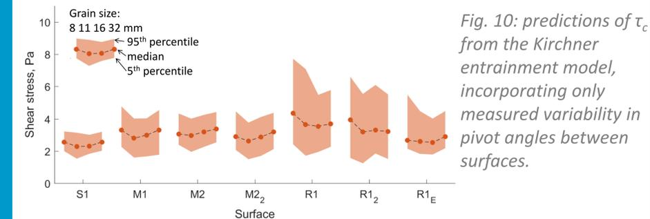
Fig. 10: predictions of  $\tau_c$  from the Kirchner entrainment model, incorporating only measured variability in pivot angles between surfaces.
