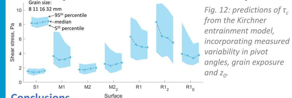
Fig. 12: predictions of  $\tau_c$  from the Kirchner entrainment model, incorporating measured variability in pivot angles, grain exposure and  $z_0$ .
