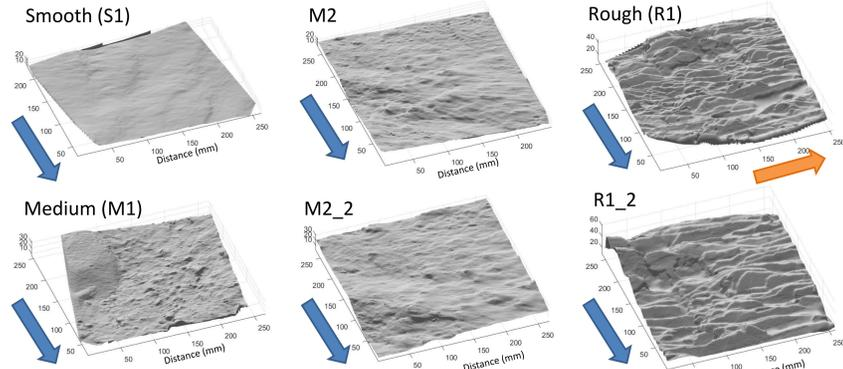
Fig. 3: The six printed surfaces. M2\_2 and R1\_2 are parts of M2 and R1 printed at twice scale. Blue arrows are pivot direction. R1 was also pivoted along orange arrow.
