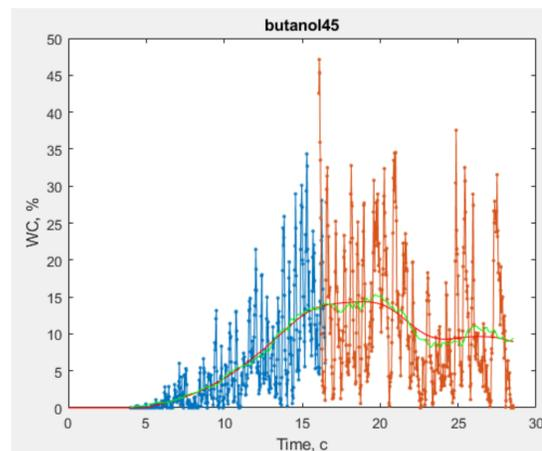
An example of obtained dependency of the part of the surface covered by whitecapping on time from wind start for fan frequency 45 Hz and water with butanol. Dotted lines – momentary values for different records. Red and green line – smoothing spline and running average, respectively.
