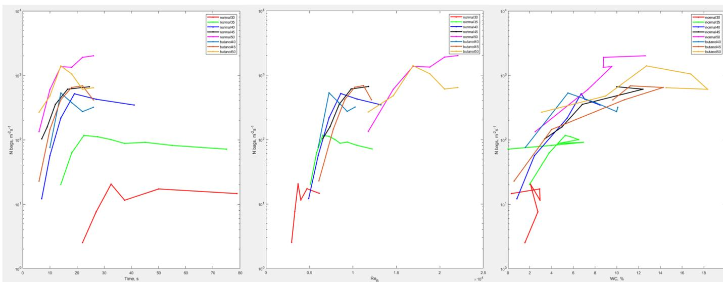
The obtained dependences of the number of bag-breakup events on time (left), on the windsea Reynolds number [Zhao et al. (2006)] (middle) and on the part of the surface covered by whitecapping (right) for different fan frequencies and the chemical composition of water.
