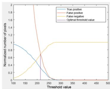
Manual marking of the wave breaking area on single frame from shadowgraph recordings of surface by a high-speed camera: the area occupied by the breaking crests of the wind waves is marked in red (left). Adaptive threshold algorithm (right): dependency of number of corresponding pixels from the selected threshold. The threshold at which the number of false positive and false negative pixels coincides is considered optimal.
