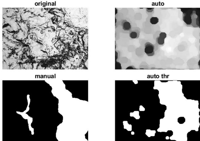
Whitecapping detection algorithm results for single frame: the original image from a high-speed camera (original), the result of preliminary image processing (auto), the result of applying the selected threshold (auto thr), manually marked areas of whitecapping on the image (manual).
