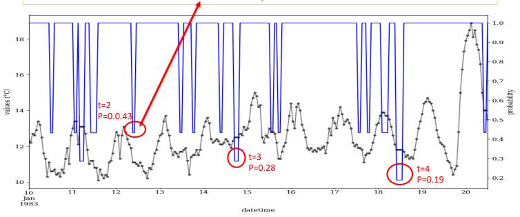
The results of performing the CVT on temperature time series at the Cape Grim station. The black and blue lines show the time series and its associated probability. The red circles highlight several constant value episodes (CVEs) with a different length (t) and probability (P). Source (EGU2020-13357) presentation.
