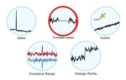
A schematic of regular data errors in a data time series. A red circle shows the focus of the developed test, i.e. constant value test (CVT). Source (EGU2020-13357) presentation.
