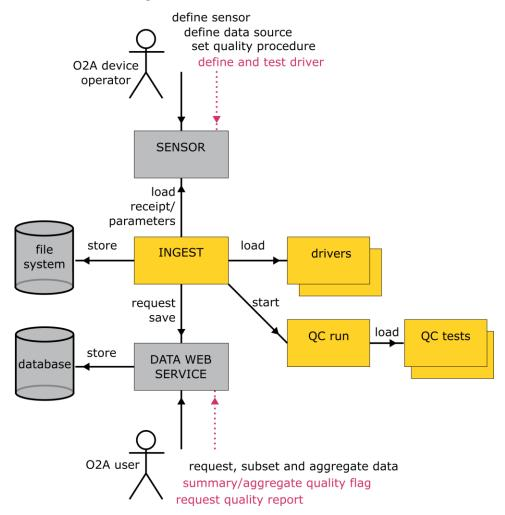
The <u>O2A-INGEST</u> performs automatic quality control to deliver quality-flagged data in the <u>O2A-DASHBOARD</u>. We use a modular approach for tests and for drivers. Drivers are used to access data at specific formats (e.g. regarding data loggers of different instruments like weather stations, buoys, ferry boxes, CTD).
