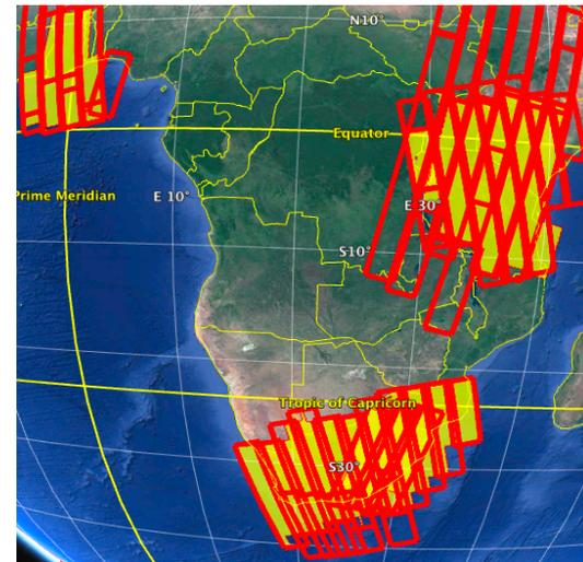
GNSS data are collected from low-cost single/dual frequency receivers: low-cost sensors can be profitably exploited in Africa where geodetic GNSS networks are missing. SAR data are collected from the Copernicus – Sentinel 1A/B mission.
