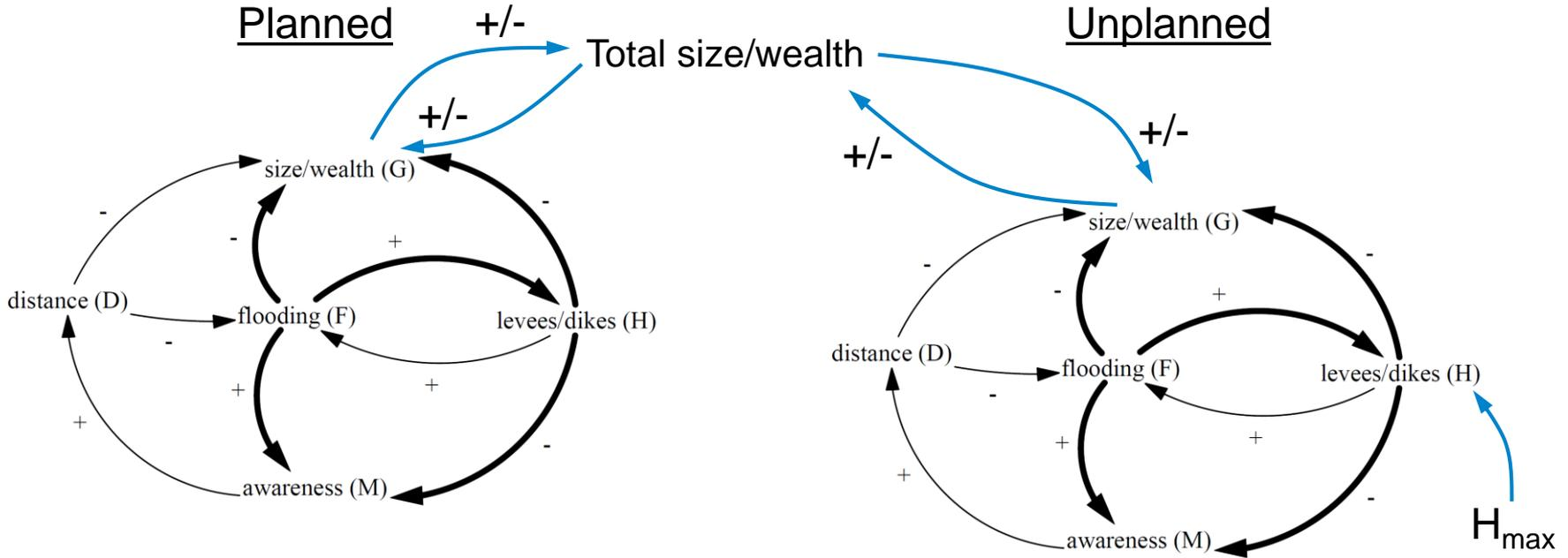
Inequality also manifests as a lack of empowerment. To account for this, we introduce a parameter,  $H_{max}$ , to limit the height of flood protection in the unplanned settlement
