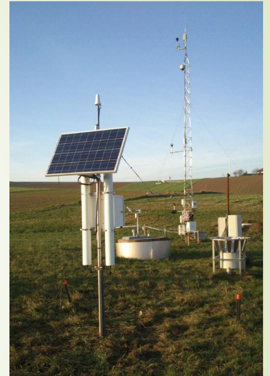
Cosmic-Ray Neutron Probe Photo taken from the paper: Franz, Trenton E., et al. "Using cosmic-ray neutron probes to monitor landscape scale soil water content in mixed land use agricultural systems." Applied and Environmental Soil Science 2016 (2016).
