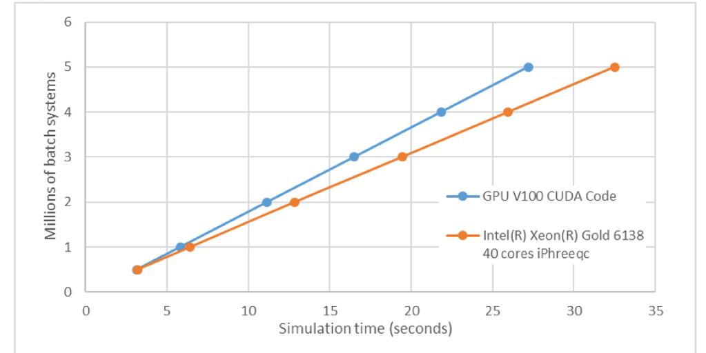
For the studied system, the CUDA code runs speciation 18% faster than the CPU OpenMP code.
