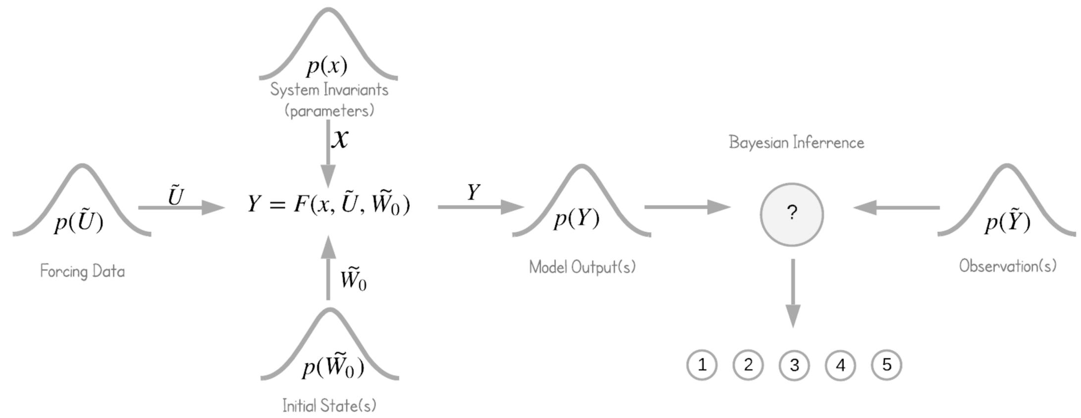
Schematic representation of data assimilation for parameter estimation, using Bayesian inference.
