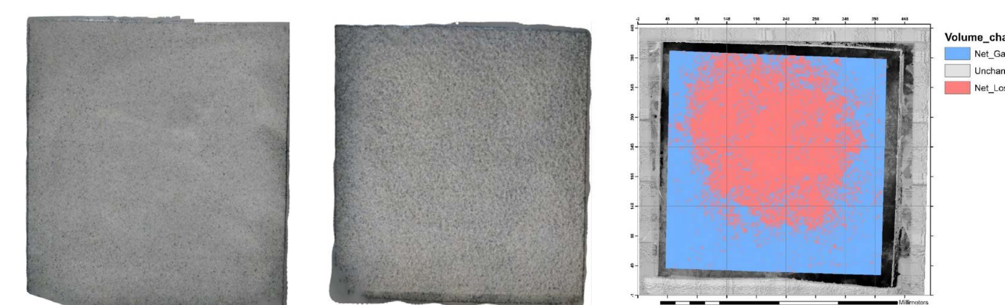
Calculated DEM before (l.) and after (m.) rainfall simulation; result of an exemplary Cut&Fill operation with ArcGIS (r.)
