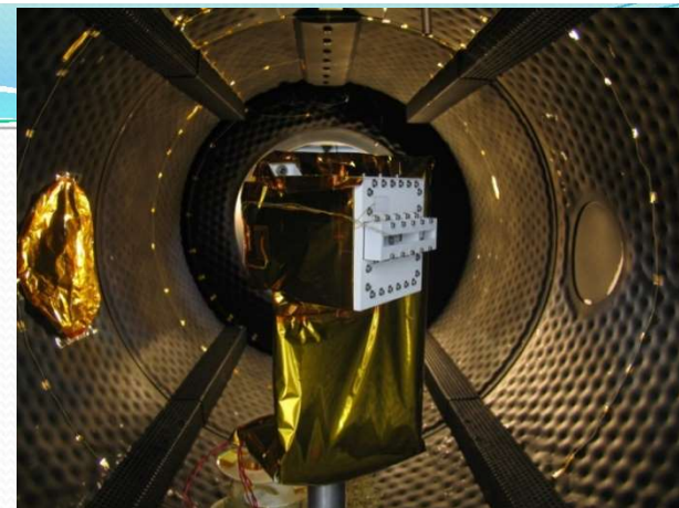
IDEE sensor STM during thermo-vacuum testing
