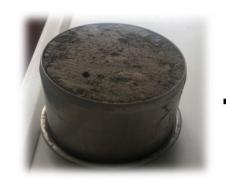
Test sample (clay, silt, sand – 100% saturated)
