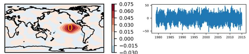
**Figure 2** First PCA-Varimax component of the preprocessed NCEP SLP dataset (1979-2014) for season DJF. We can derive a time series for each component.
