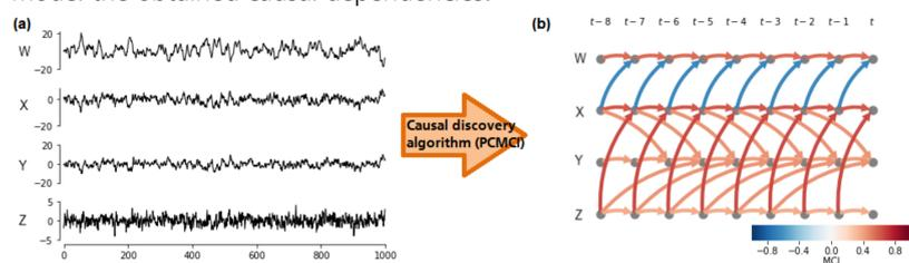
**Figure 3** Example of an application of PCMCI (Runge et al., 2019). (a) Simulated time series of four variables linked by time-lagged linear dependencies. (b) Output graph of the PCMCI Causal Discovery algorithm exhibiting found time-lagged dependencies and their strengths.
