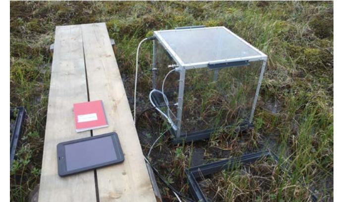
Small-scale CH<sub>4</sub> flux measurements by transparent closed chambers and an Ultraportable Greenhouse Gas Analyzer (UGGA 30-p, Los Gatos Research)
