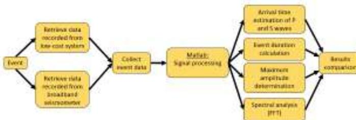
Figure 4: The workflow concerning the steps followed for each seismic event during this study.
