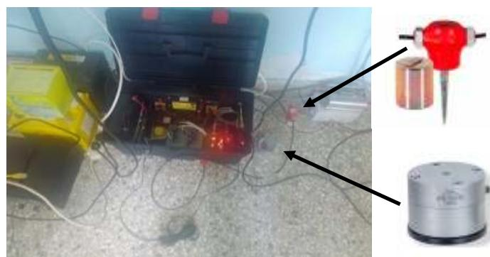
Figure 3. View of the installed low cost seismometer (black case) along with the broad band seismometer in the area of Evgiros (Lefkada island). In addition are shown: a) Velocity sensor used (Geophone GS1D – 4.5 Hz) and b) acceleration sensor used (Accelerometer KB12VD).
