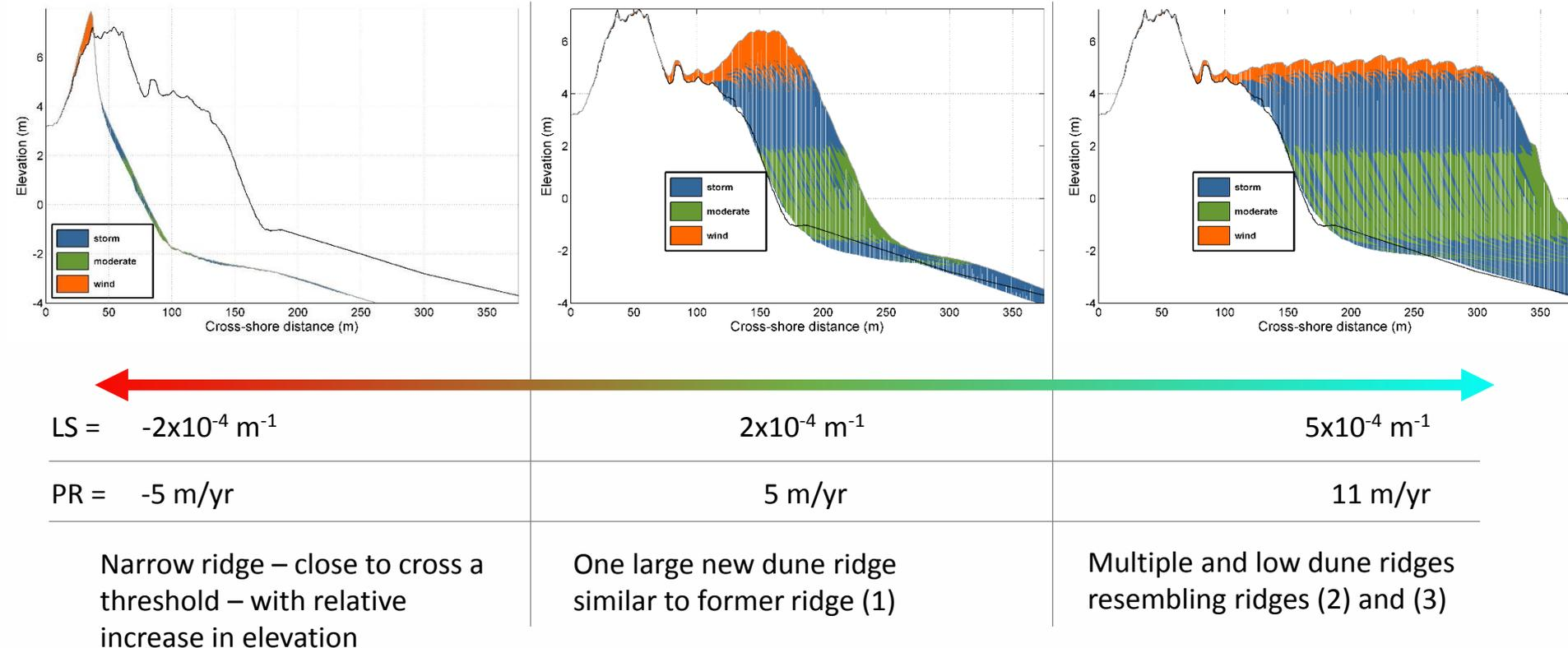
\*The calibration of modelling parameters was done using the evolution of the profile observed between 2009 and 2011. Simulations used the same parameters and the schematized meteocean conditions between 2009 and 2011 repeated 10 times to simulate 20 years of change
