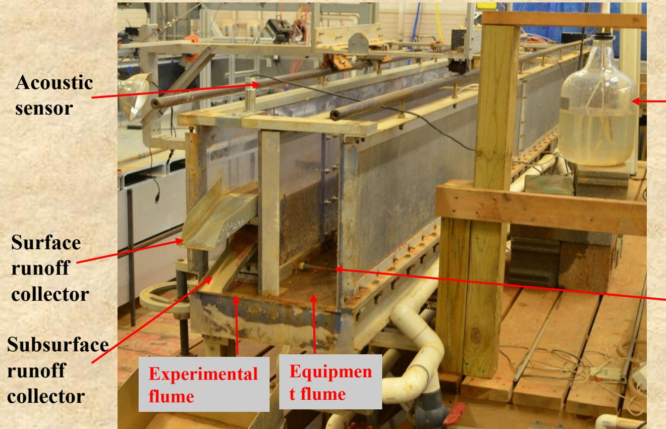
**Ability to sample overland flow and pipeflow separately at outlet and to apply a perched water table or free-drainage conditions**
