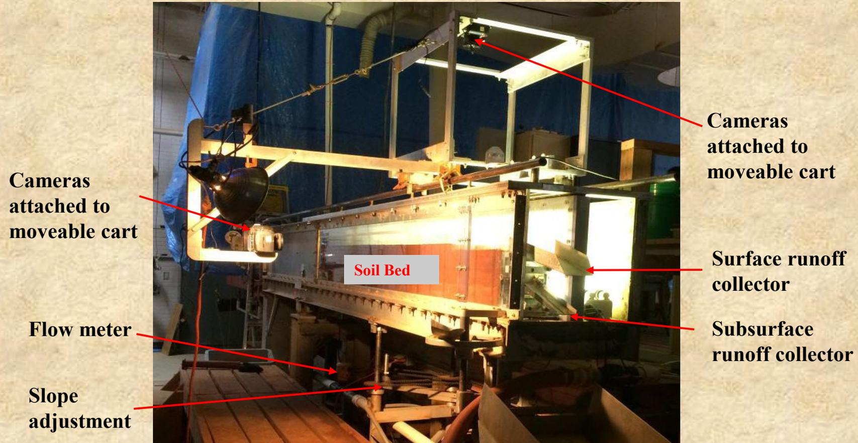
**Soil pipe created below the surface and headcut on surface. Ability to track changes in headcut plunge pool morphology and headcut advance by cameras**
