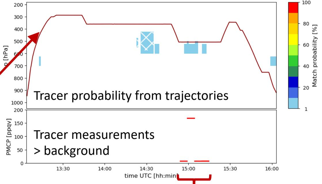
Vertical cross section of the tracer flight (red line) "through" WCB probability
